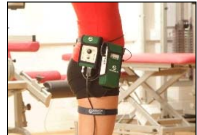
Depending on the need, the Multi-Mode FootSwitch System may be connected to the Telemyo G2 Transmitter "Digital In" or EMG ports.
