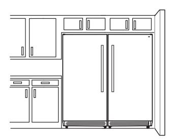
IMPORTANT: Do not install the appliances near an oven, radiator, or other heat source, nor in a location where the temperature will fall below 40°F (5°C).
