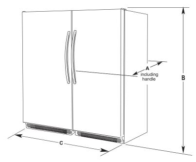
Width "C" includes recommended spacing (0.25 in.) between refrigerator and freezer
